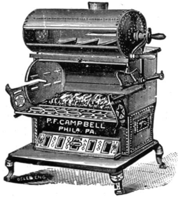
FIGURE 46.2. Hand-turned cylindrical bean roaster. Source: P. F. Campbell, 1900. Courtesy of Rodney Snyder. (Used with permission.)
